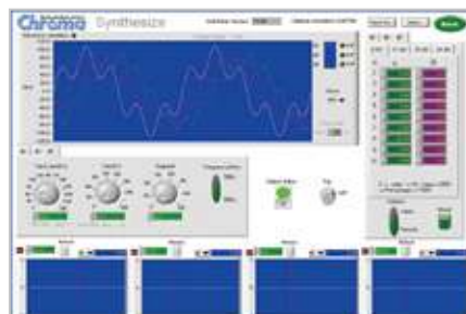
Distorted Waveform Editor
